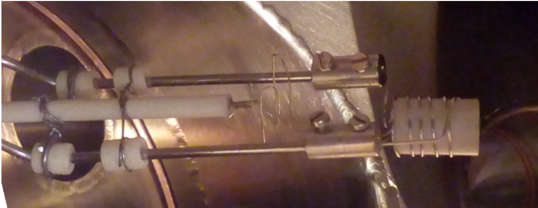
Figure B.1.: Ga evaporator used for the deposition of Ga onto Au surfaces. Used is an Al 2 O 3 crucible of 8 mm inner- and 10 mm outer diameter, which is fitted into a solenoid from tungsten wire of 0.5 mm diameter. Crucible temperature was measured using a type K thermocouple pressed to the outer bottom of the crucible. Typically powers to achieve crucible temperatures above 800 K exceeded 10 · 12 V A.
