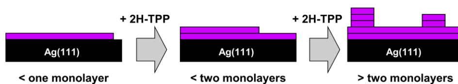
Figure 14: Scheme of the initial stages of 2H-TPP film growth on Ag(111) at temperatures between 80 and 315 K. The growth behavior on Au(111) is identical. 84
