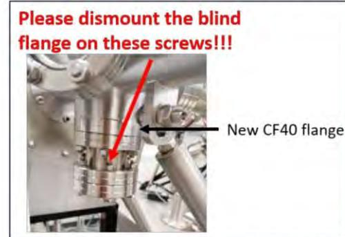
Fig. 26: Dismounting the blind flange of the FEL chamber on the DASSA.
