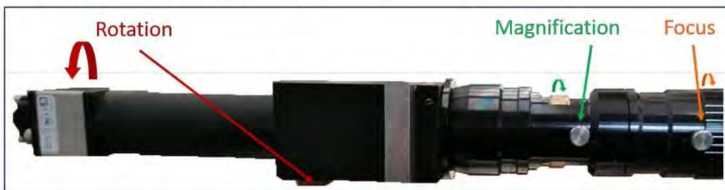
Fig. 18: Camera setup with rotation, magnification and focus screws.
