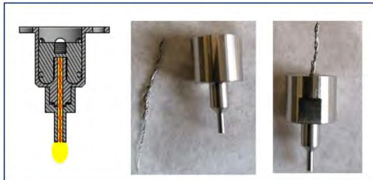
**Figure S2:** Left: Schematic representation of the twisted wires in the cannula, middle: Photo of the twisted wires and the cannula and right: Photo of the twisted wires inserted into the cannula.
