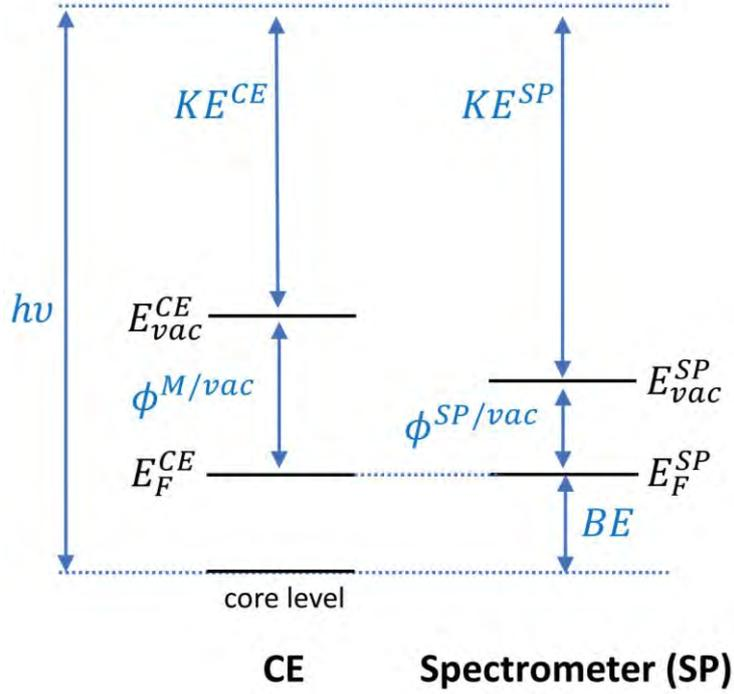
Figure 7 Energy diagrams depicting the potential of metallic CE and spectrometer.
