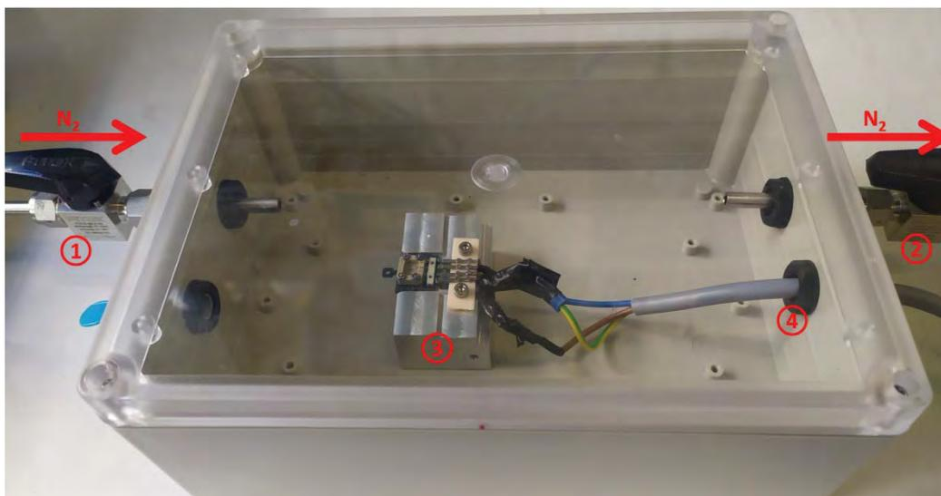
*Figure 38 Air-tight box used to perform the measurements in  $N_2$  atmosphere and air (numbers, see text).*
