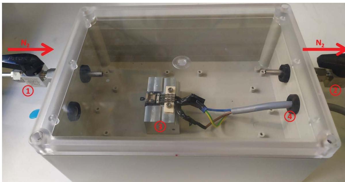
Figure A29 Air-tight box used to perform the measurements in  $N_2$  atmosphere and air (numbers, see text).
