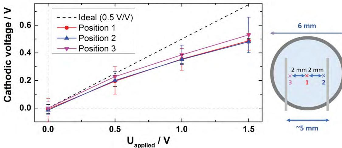
Figure A2 (Left) Cathodic voltage of  $[C_1C_1Im][Tf_2N]$  at different probing positions between Pt electrodes. (Right) Schematic sketch of XPS probing positions. In case of an ohmic drop between the electrodes, the potential of the IL should change depending on the position, with the XPS peak shifting accordingly. Our data show that the XP peaks did not change depending on the probing positions, which implies that no ohmic drop exists between the electrodes.
