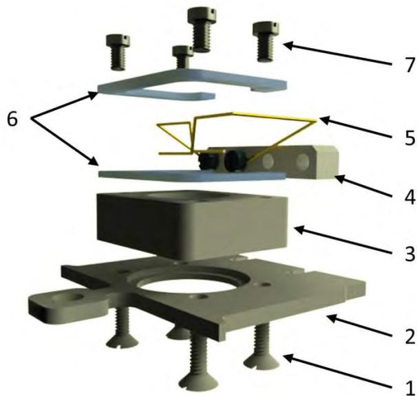
Figure 12 (left) Photo of the electrochemical cell used in this thesis; (right) Explosion drawing of the electrochemical cell showing all its components (numbers, see text).
