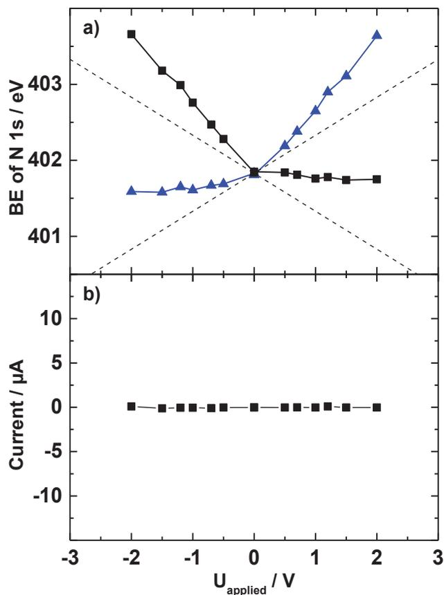
Figure A20 (a) Data for [C<sub>8</sub>C<sub>1</sub>Im][Tf<sub>2</sub>N]<sub>x</sub>Cl<sub>1-x</sub> (x = 0) on Au. (b) Residual current during the XPS measurements at constant external voltages applied.
