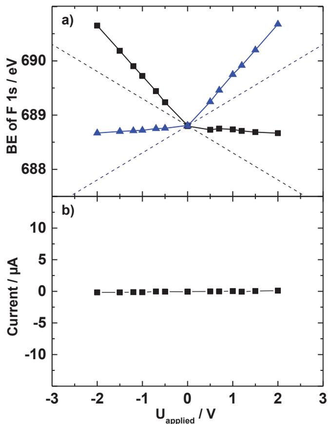
Figure A15 (a) Data for [C<sub>8</sub>C<sub>1</sub>Im][Tf<sub>2</sub>N]<sub>x</sub>Cl<sub>1-x</sub> (x = 0.99) on Au. (b) Residual current during the XPS measurements at constant external voltages applied.
