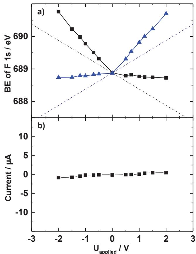
Figure A18 (a) Data for [C<sub>8</sub>C<sub>1</sub>Im][Tf<sub>2</sub>N]<sub>x</sub>Cl<sub>1-x</sub> (x = 0.1) on Au. (b) Residual current during the XPS measurements at constant external voltages applied.
