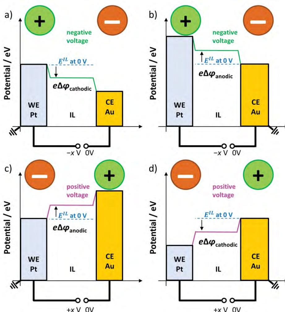
Figure 47 Schematic representation of the IL/electrodes interfaces for negative (a and b) and positive (c and d) polarization with the Pt WE grounded (a and c) and the Au CE grounded (b and d); cations and anions at the electrodes are represented as green and orange circles respectively.
