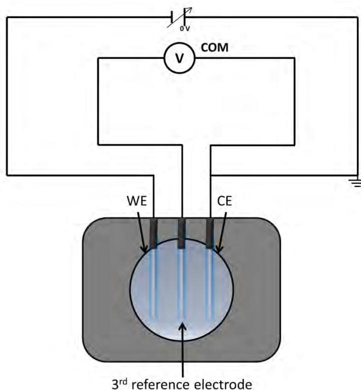
*Figure A28 Sketch of the electrochemical cell used for the potential screening measurements in  $N_2$  and air.*
