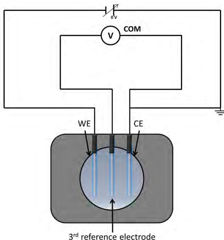
Figure 40 Sketch of the electrochemical cell used for the potential screening measurements in  $N_2$  and air.
