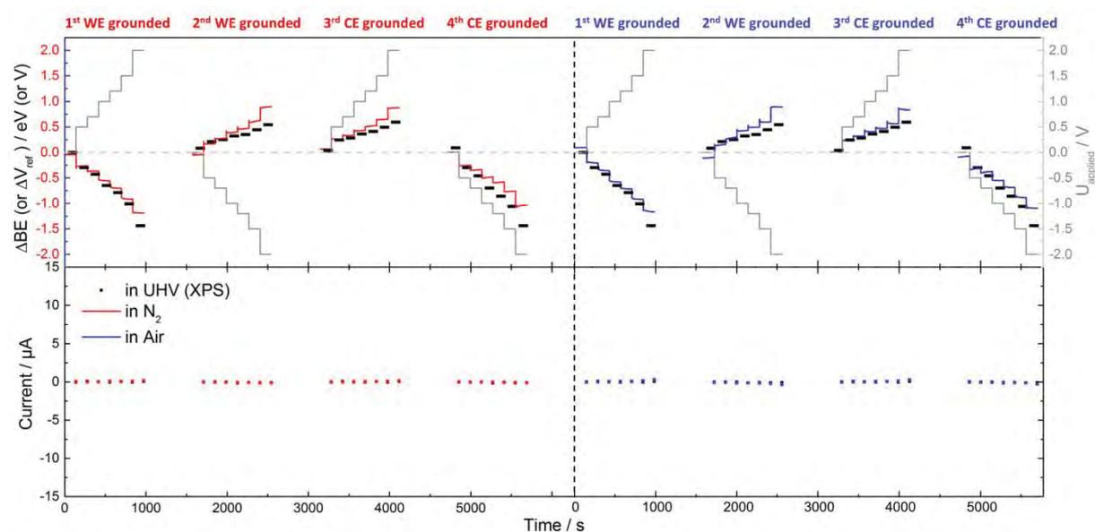
Figure A33 Top: Time-dependent measurement of PS curves of [C<sub>8</sub>C<sub>1</sub>Im][Tf<sub>2</sub>N] with Pt electrodes recorded in UHV by XPS (black), N<sub>2</sub> atmosphere (red) and air (blue). The applied voltage profiles are shown as grey traces. Bottom: Averaged current recorded during the measurements for [C<sub>8</sub>C<sub>1</sub>Im][Tf<sub>2</sub>N] with Pt electrodes.
