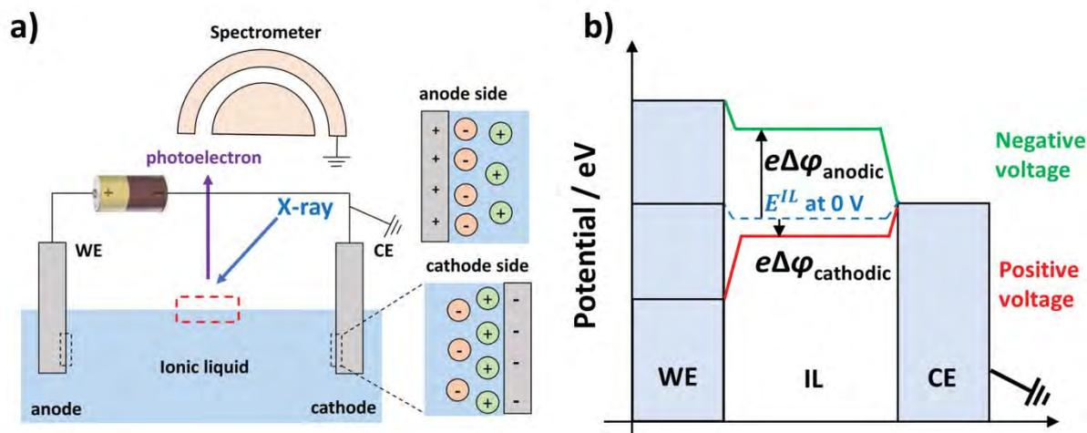
Figure 22 a) Schematic figure of our experimental setup and the charged interfaces with the CE grounded. b) Potential diagram of IL and electrodes with an applied positive (red) or negative (green) potential. The potential drops at the WE/IL and CE/IL interfaces are indicated as  $\Delta\phi_{\text{anodic}}$  and  $\Delta\phi_{\text{cathodic}}$ , respectively, according to the polarity of the electrodes.
