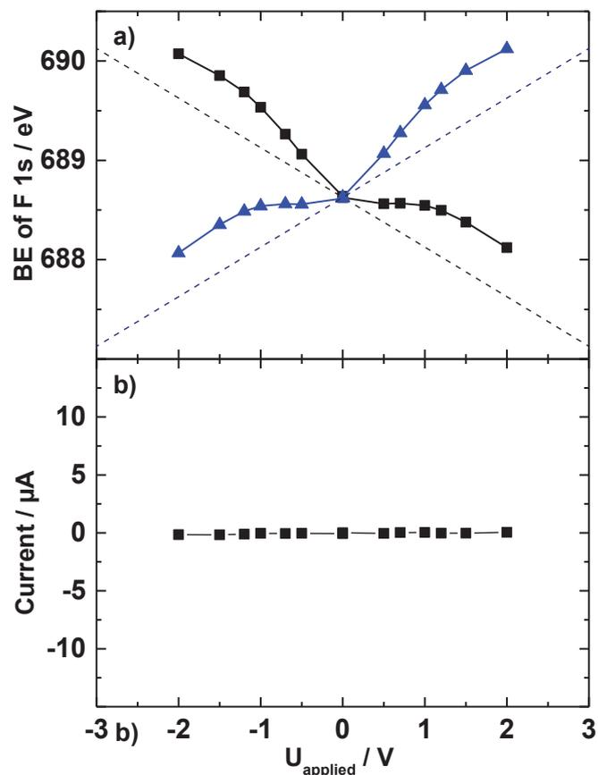
Figure A14 (a) Data for [C<sub>8</sub>C<sub>1</sub>Im][Tf<sub>2</sub>N]<sub>x</sub>Cl<sub>1-x</sub> (x = 0.999) on Au. (b) Residual current during the XPS measurements at constant external voltages applied.
