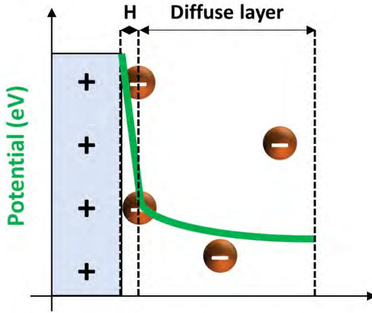
Figure 3 Schematic representation of the Gouy-Chapman-Stern EDL model and the variation in potential according to the distance from the electrode.
