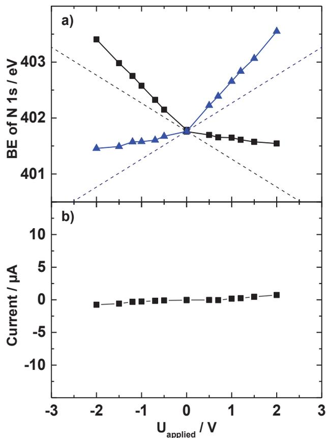
Figure A19 (a) Data for [C<sub>8</sub>C<sub>1</sub>Im][Tf<sub>2</sub>N]<sub>x</sub>Cl<sub>1-x</sub> (x = 0.01) on Au. (b) Residual current during the XPS measurements at constant external voltages applied.
