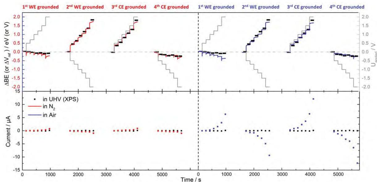
Figure A30 Top: Time-dependent measurement of PS curves of [C<sub>8</sub>C<sub>1</sub>Im]Cl with Au electrodes recorded in UHV by XPS (black), N<sub>2</sub> atmosphere (red) and air (blue). The applied voltage profiles are shown as grey traces. Bottom: Averaged current recorded during the measurements for [C<sub>8</sub>C<sub>1</sub>Im]Cl with Au electrodes.
