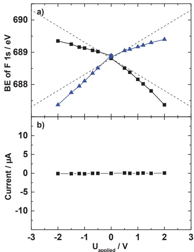
Figure A21 (a) Data for [C<sub>8</sub>C<sub>1</sub>Im][Tf<sub>2</sub>N]<sub>x</sub>Cl<sub>1-x</sub> (x = 1.0) on Pt. (b) Residual current during the XPS measurements at constant external voltages applied.
