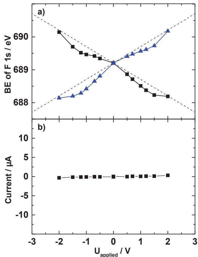
Figure A24 (a) Data for [C<sub>8</sub>C<sub>1</sub>Im][Tf<sub>2</sub>N]<sub>x</sub>Cl<sub>1-x</sub> (x = 0.5) on Pt. (b) Residual current during the XPS measurements at constant external voltages applied.
