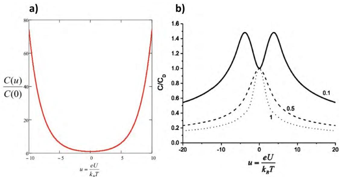
Figure 5 a) U-shape capacitance curve predicted by the Gouy-Chapman EDL model; b) Capacitance curves predicted by the Kornyshev EDL model showing bell and camel shapes for large and small values of  $\gamma$  respectively. (Adapted with permission from M. V. Fedorov, A. A. Kornyshev, Ionic liquids at electrified interfaces. *Chem. Rev.* **2014**, 114, 2978-3036. Copyright 2014 American Chemical Society).
