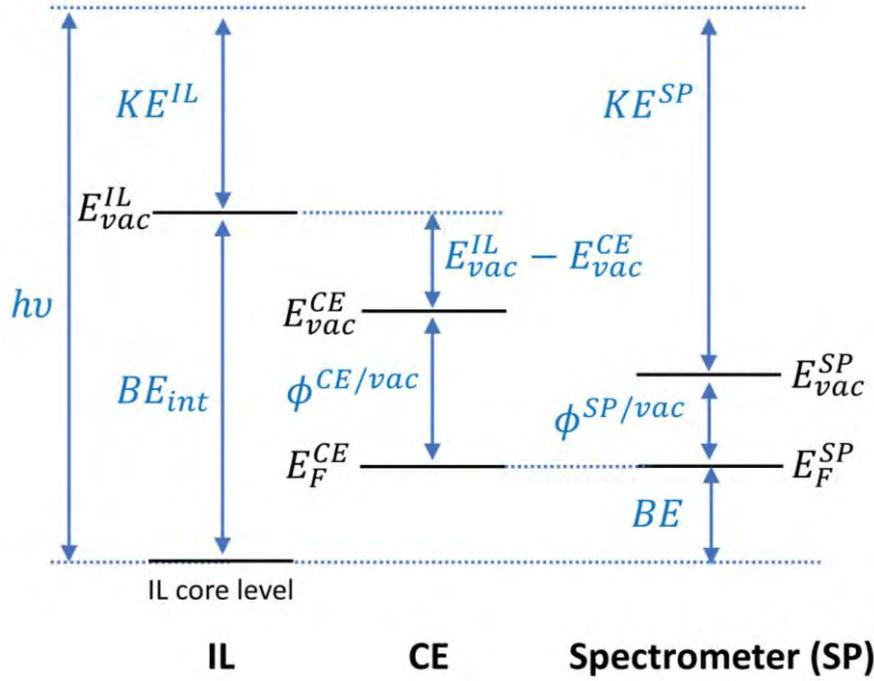
Figure 8 Energy diagrams depicting the potential of IL, metallic CE and spectrometer.
