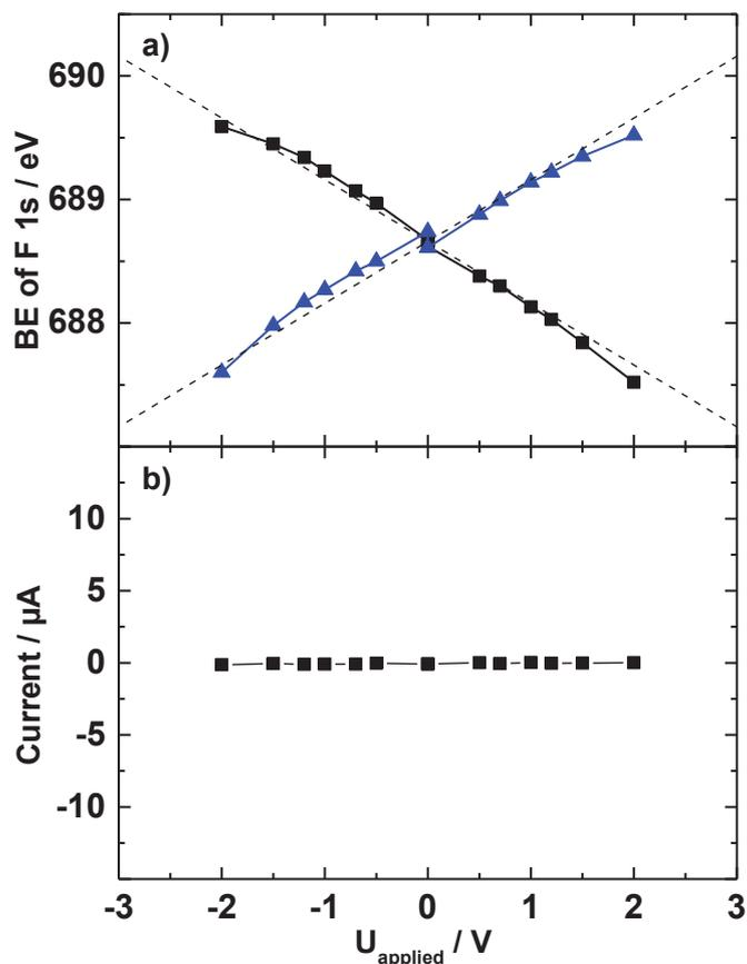
Figure A13 (a) Data for [C<sub>8</sub>C<sub>1</sub>Im][Tf<sub>2</sub>N]<sub>x</sub>Cl<sub>1-x</sub> (x = 1) on Au. (b) Residual current during the XPS measurements at constant external voltages applied.
