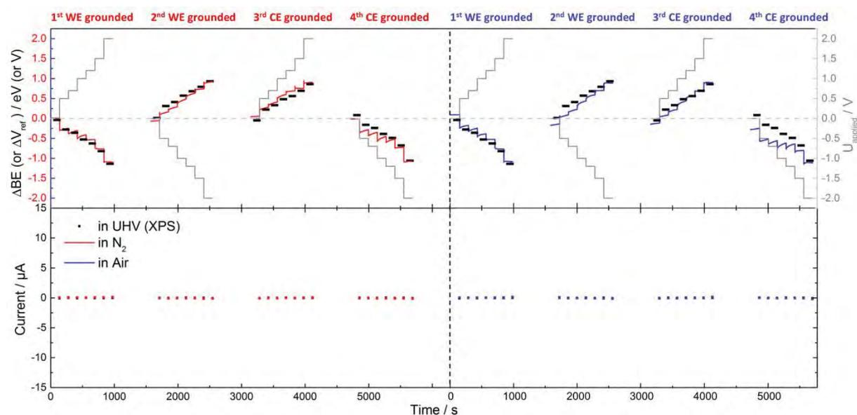
Figure A32 Top: Time-dependent measurement of PS curves of [C<sub>8</sub>C<sub>1</sub>Im][Tf<sub>2</sub>N] with Au electrodes recorded in UHV by XPS (black), N<sub>2</sub> atmosphere (red) and air (blue). The applied voltage profiles are shown as grey traces. Bottom: Averaged current recorded during the measurements for [C<sub>8</sub>C<sub>1</sub>Im][Tf<sub>2</sub>N] with Au electrodes.
