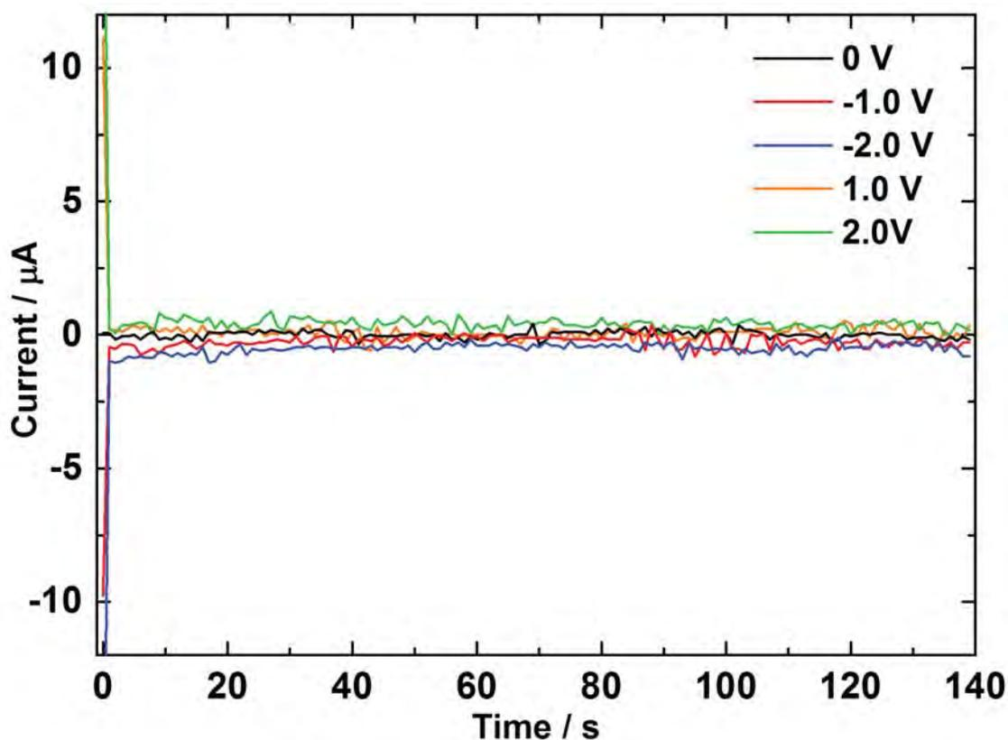
Figure A12. Current between Au electrodes in  $[C_8C_1Im][Tf_2N]_xCl_{1-x}$  ( $x = 0.01$ ) with a constant applied potential. The charging current for an EDL formation decreased rapidly within 1 s. All XPS measurements were started after the EDL formation and the residual current during the measurement was less than  $0.2 \mu A$ ; note that for this specific cell a residual leakage current of  $\pm 0.4 \mu A$  was present at the highest voltage of  $\pm 2V$ .
