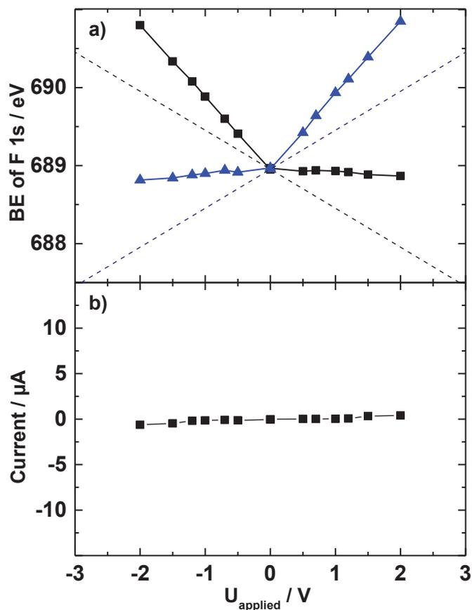
Figure A16 (a) Data for [C<sub>8</sub>C<sub>1</sub>Im][Tf<sub>2</sub>N]<sub>x</sub>Cl<sub>1-x</sub> (x = 0.9) on Au. (b) Residual current during the XPS measurements at constant external voltages applied.
