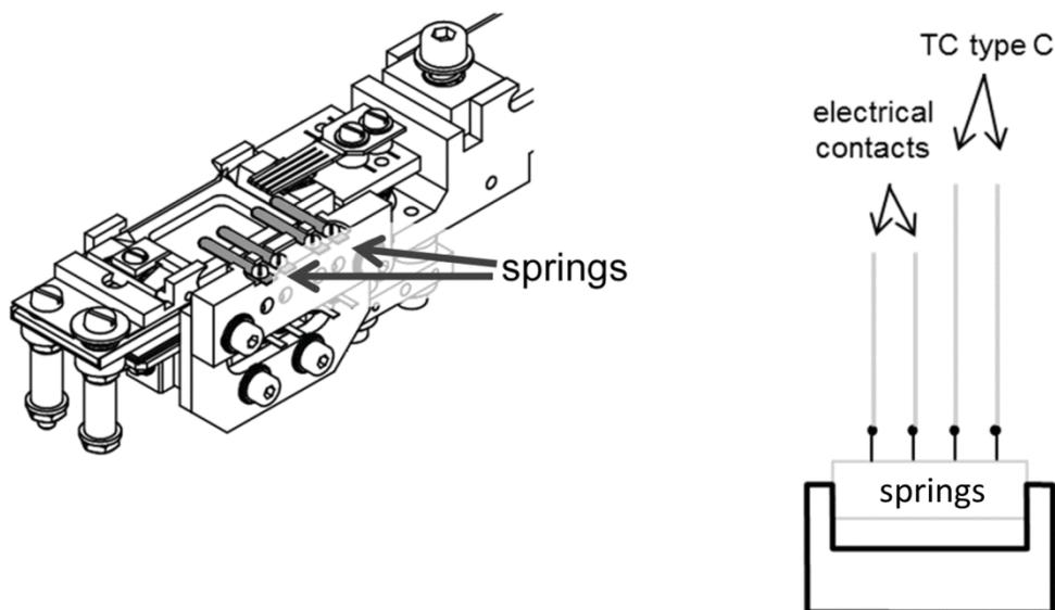
Figure 13 (left) Sketch of the sample stage of DASSA instrument with its four contact springs; (right) sketch of electrical contacts and thermocouples springs.
