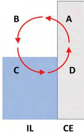
Figure 9 Schematic representation of solid/vacuum, vacuum/liquid, liquid/solid interface and the energies involved to move an electron across them (letters, see text).
