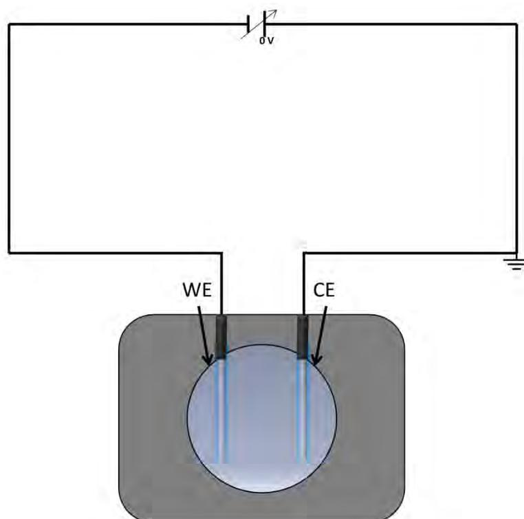
Figure 6 Sketch of the electrochemical cell used for PS measurements.
