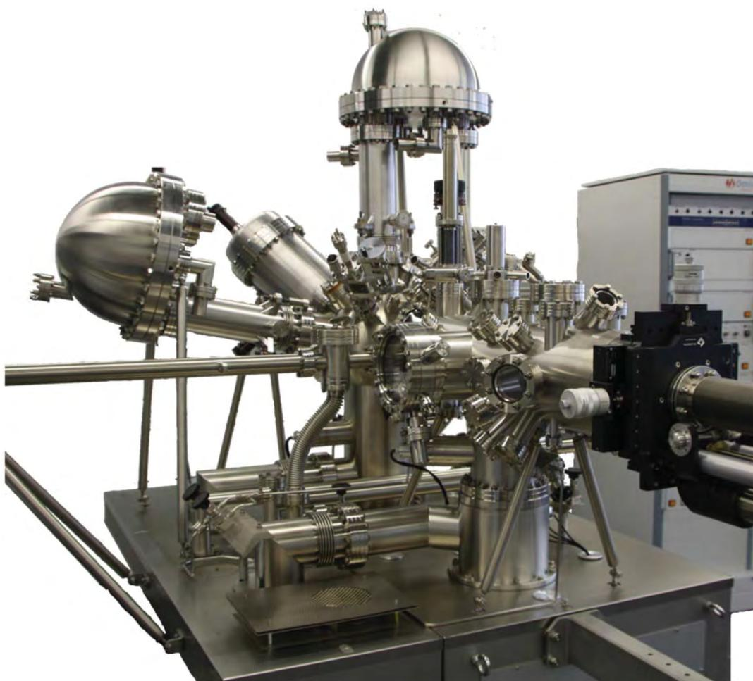
*Figure 10 Photo of the UHV-based XPS chamber (DASSA) used in this thesis.*
