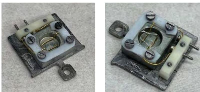
Figure A1 Electrochemical cell used for the potential screening measurements before filling IL (left) and after filling IL (right).
