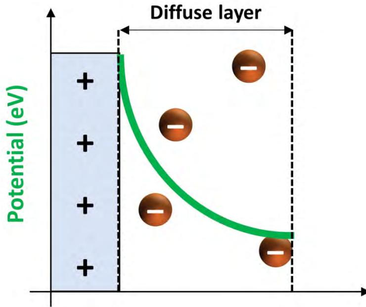
Figure 2 Schematic representation of the Gouy-Chapman EDL model and the variation in potential according to the distance from the electrode.
