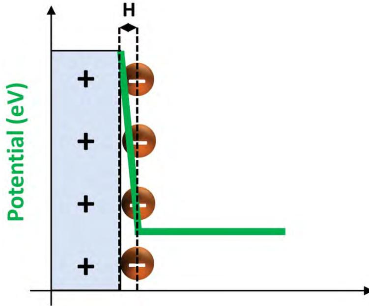
Figure 1 Schematic representation of the Helmholtz EDL model and the variation in potential according to the distance from the electrode.
