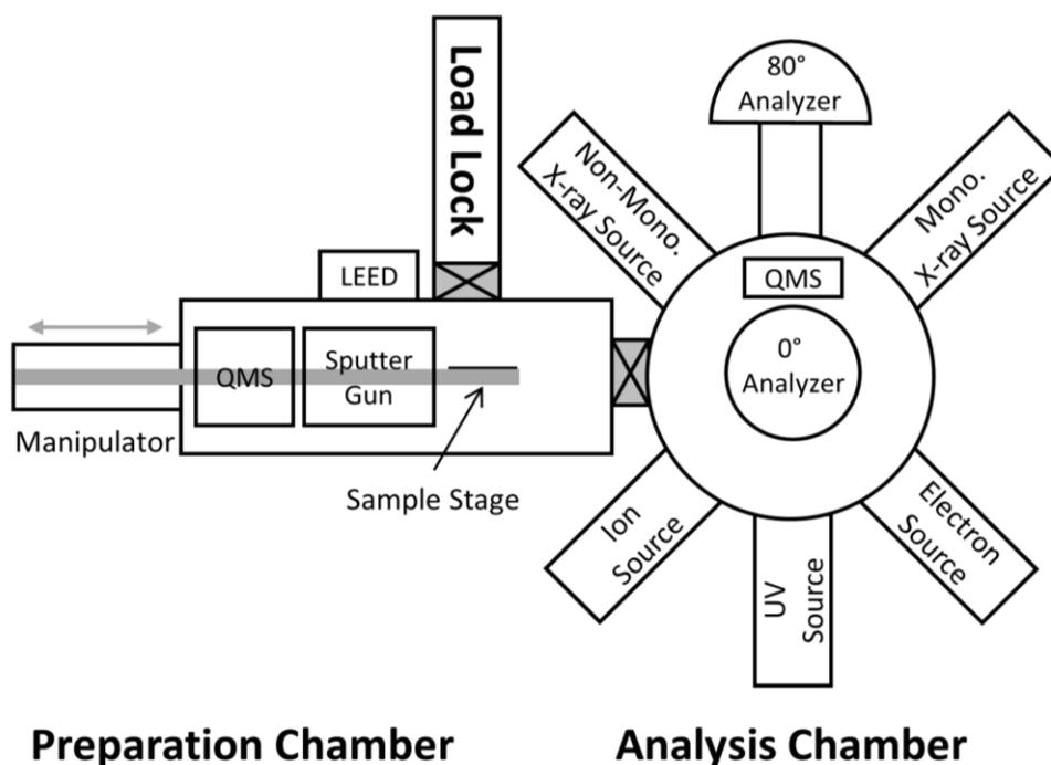
Figure 11 Schematic representation of DASSA.
