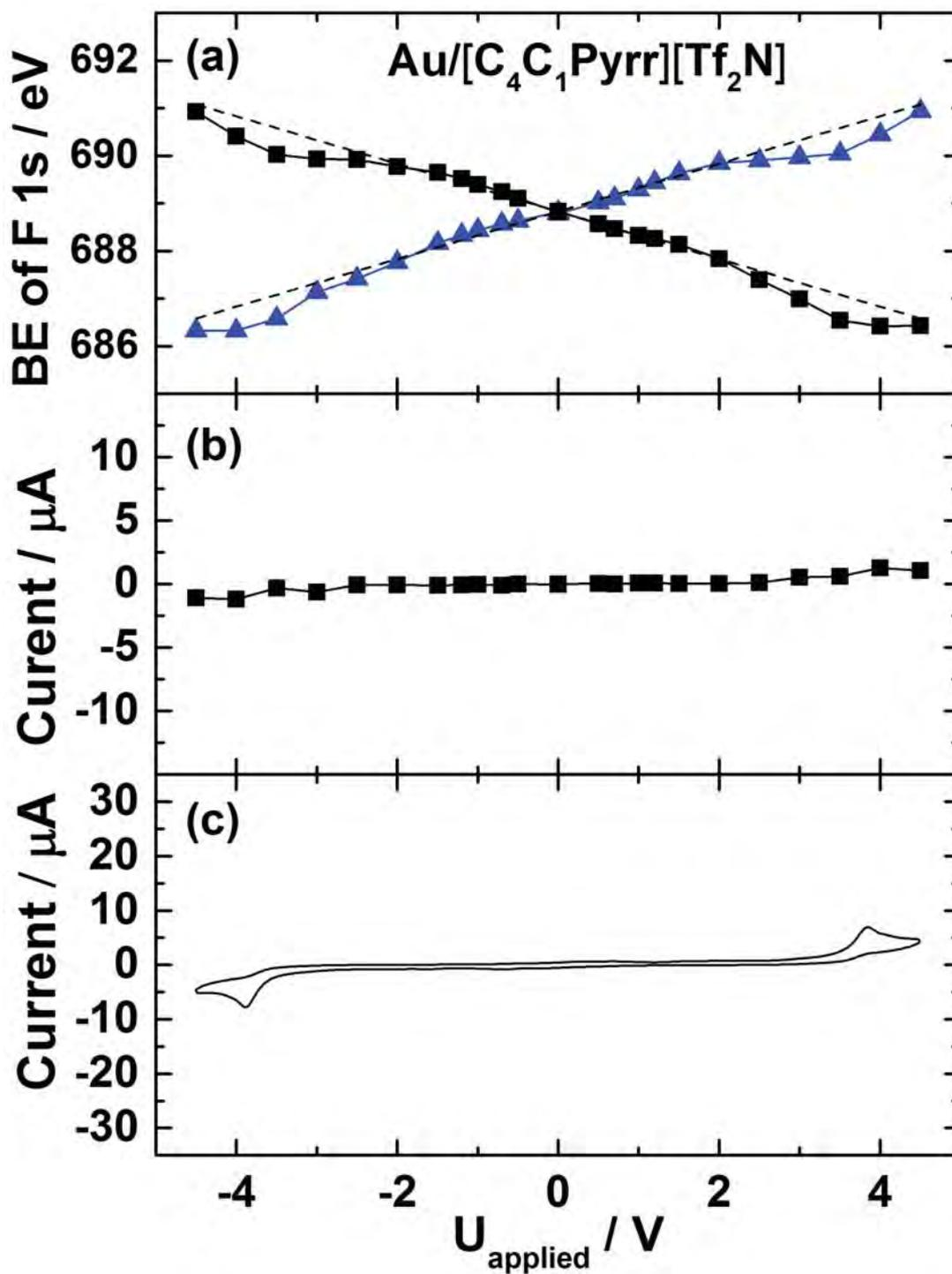
Figure A11 (a) BE of F 1s in  $[\text{C}_4\text{C}_1\text{Pyrr}][\text{Tf}_2\text{N}]$  XPS spectra according to  $U_{\text{applied}}$  in the cases of an Au WE-grounded ( $d=0.25$  mm) (black square) and an Au CE-grounded ( $d=0.25$  mm) (blue triangle) setups. The ideal lines are indicated as dashed lines. (b) Residual current at a constant  $U_{\text{applied}}$  during the XPS measurement. (c) Potential sweep measurement. The ramping rate is 50 mV/s.
