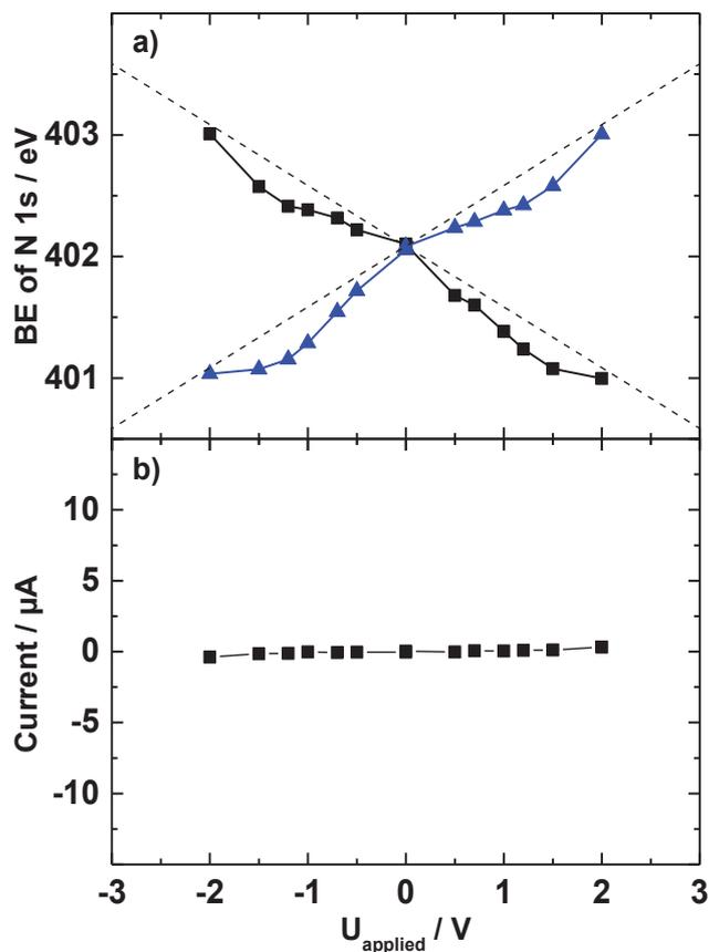
Figure A25 (a) Data for [C<sub>8</sub>C<sub>1</sub>Im][Tf<sub>2</sub>N]<sub>x</sub>Cl<sub>1-x</sub> (x = 0.1) on Pt. (b) Residual current during the XPS measurements at constant external voltages applied.
