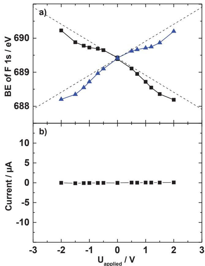
Figure A22 (a) Data for [C<sub>8</sub>C<sub>1</sub>Im][Tf<sub>2</sub>N]<sub>x</sub>Cl<sub>1-x</sub> (x = 0.99) on Pt. (b) Residual current during the XPS measurements at constant external voltages applied.
