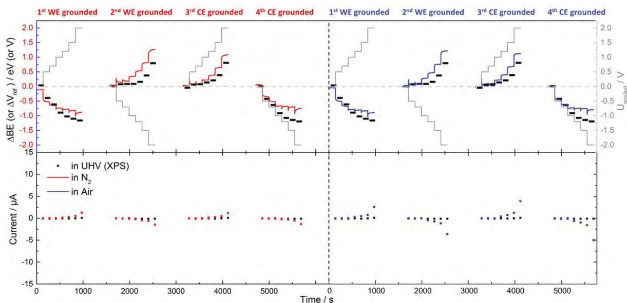
Figure A31 Top: Time-dependent measurement of PS curves of [C<sub>8</sub>C<sub>1</sub>Im]Cl with Pt electrodes recorded in UHV by XPS (black), N<sub>2</sub> atmosphere (red) and air (blue). The applied voltage profiles are shown as grey traces. Bottom: Averaged current recorded during the measurements for [C<sub>8</sub>C<sub>1</sub>Im]Cl with Pt electrodes.
