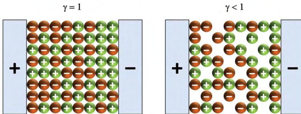
Figure 4 Schematic representation of the lattice saturation parameter for an IL between two polarized electrodes. (Adapted with permission from M. V. Fedorov, A. A. Kornyshev, Ionic liquids at electrified interfaces. *Chem. Rev.* **2014**, 114, 2978-3036. Copyright 2014 American Chemical Society).
