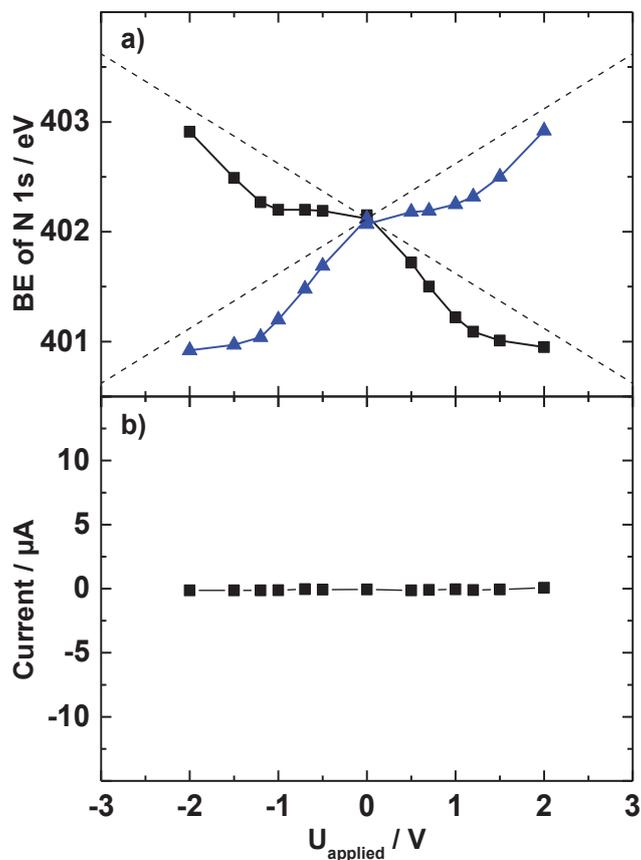
Figure A27 (a) Data for  $[C_8C_1Im][Tf_2N]_xCl_{1-x}$  ( $x = 0$ ) on Pt. (b) Residual current during the XPS measurements at constant external voltages applied.
