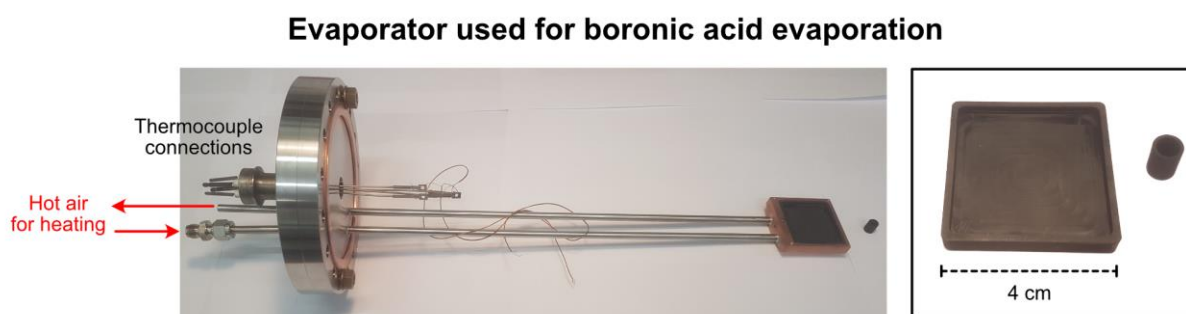
Figure 27: Picture of the evaporator used to evaporate boronic acids (left). Since the large surface area and close proximity to the sample enable comparatively low evaporation temperatures, it is sufficient to heat this evaporator with hot air. A direct comparison of the carbon crucibles of this evaporator and our standard evaporators (right) illustrates the massive difference in surface area of 16 \text{ cm}^2 and 0.3 \text{ cm}^2 .
